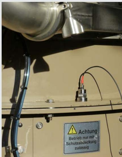
**"Hearing aid":** A computer program recognizes, via a microphone attached to the seed treatment tank, the exact time when the seed treatment process must stop.
